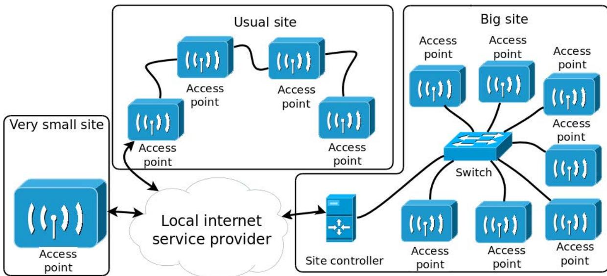
In very small sites off the shelf wireless routers running IUNGO provided custom firmware will be directly connected to local internet service provider. A selected set of the wireless router models will be supported by custom firmware to act as IUNGO network compatible access points. For
